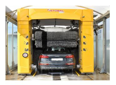
The ISTOBAL FLEX5 car wash with three brushes has been chosen for its advanced wash and dry technology and its high technical reliability. Bosch Car Service Kleverlaan has this model in its largest version so the machine can wash company buses up to 2.70 meters high and pick-up trucks up to 2.50 meters wide. This allows the car service company to offer the wash service to a wider range of vehicles that come to its facilities daily.
